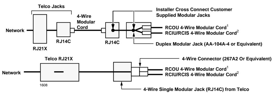
1. 4-wire modular jacks such as graybar part number AA-104A-4 could be used in place of the two modular jacks; or, a T-connector such as graybar part number 267A2 Adaptor could be used as shown below:
