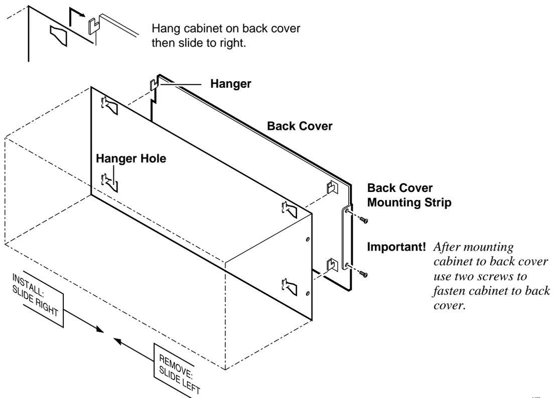
Figure 5-8 DK424 Mounting Cabinet on Back Cover
