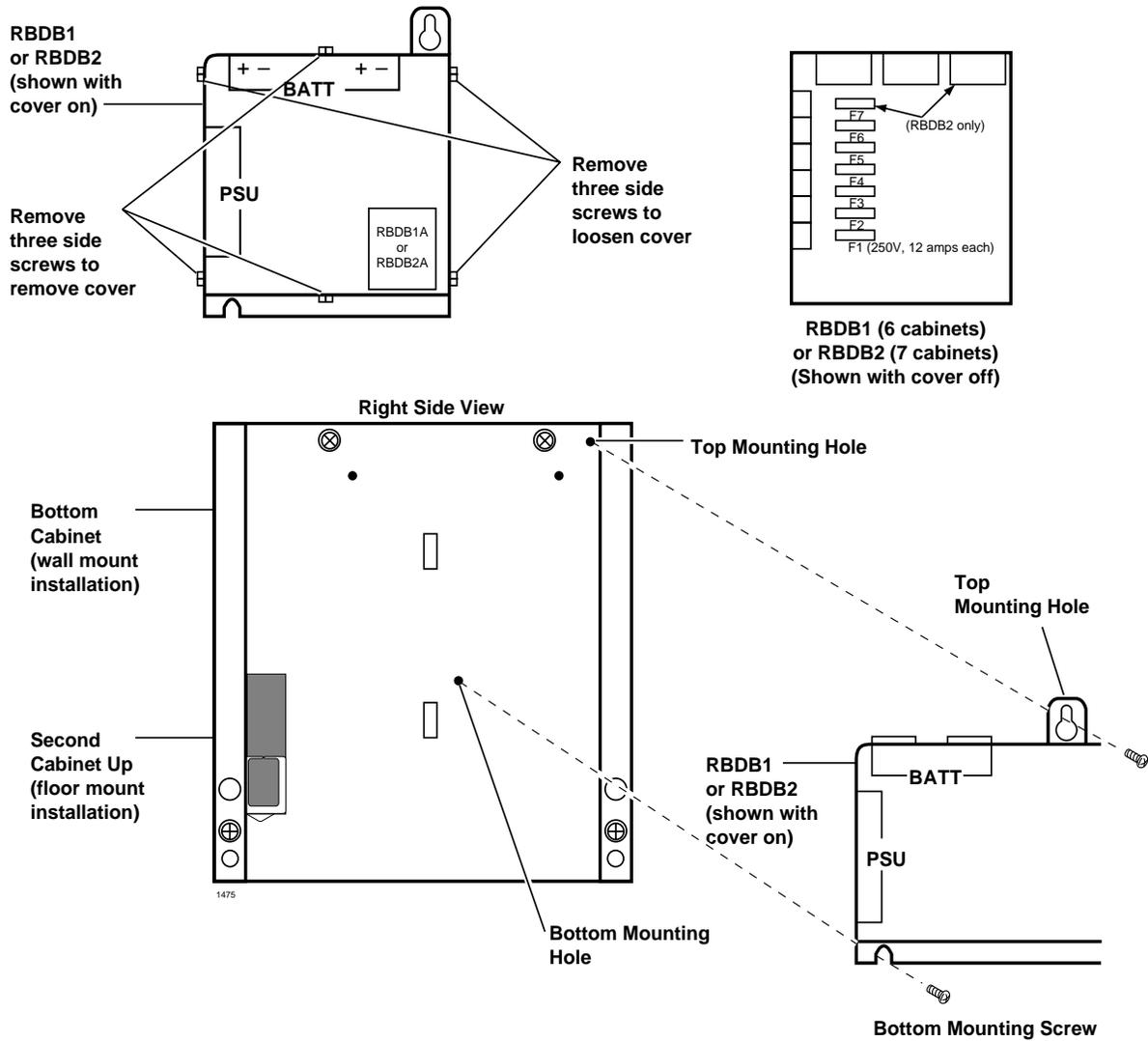
Figure 5-23 Battery Distribution Box (RBDB) Installation
