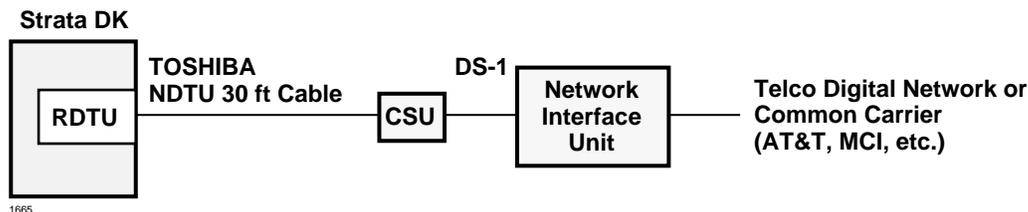
Figure 6-4 RDTU Connection to Digital Network or OCC
