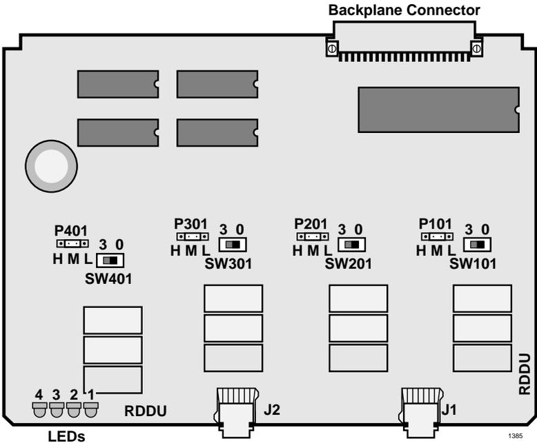
**Figure 7-18 RDDU Controls, Indicators, and Interface Connectors**
