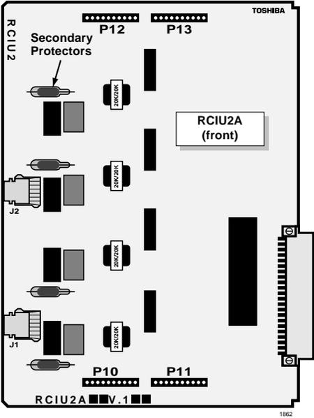
Figure 7-12 DK40i RCIU2 PCB Installation
