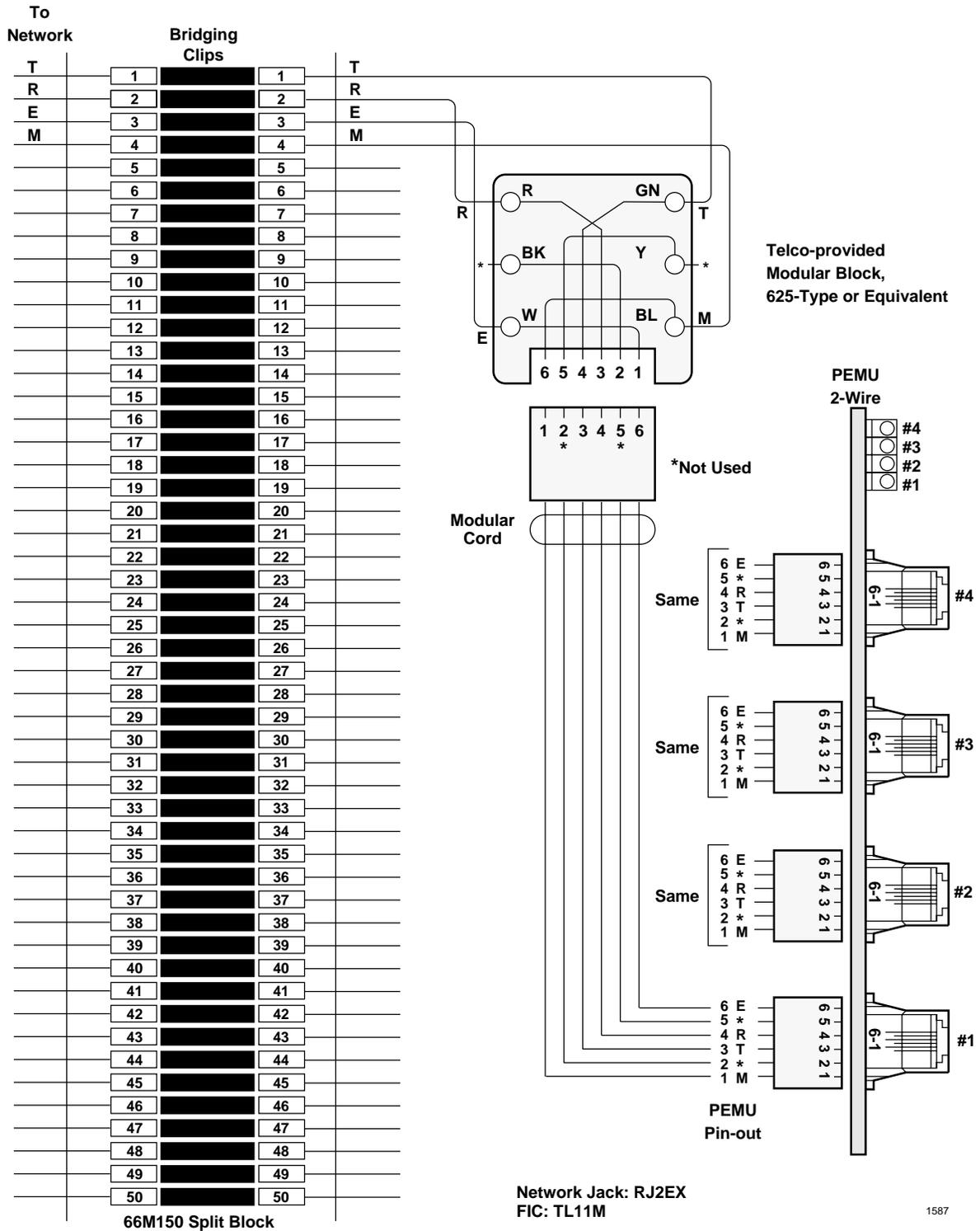
Figure 8-30 MDF Wiring/2-Wire Tie Line to PEMU
