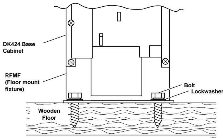
**Figure 5-17 Floor Mount Installation – Wooden Floor**
