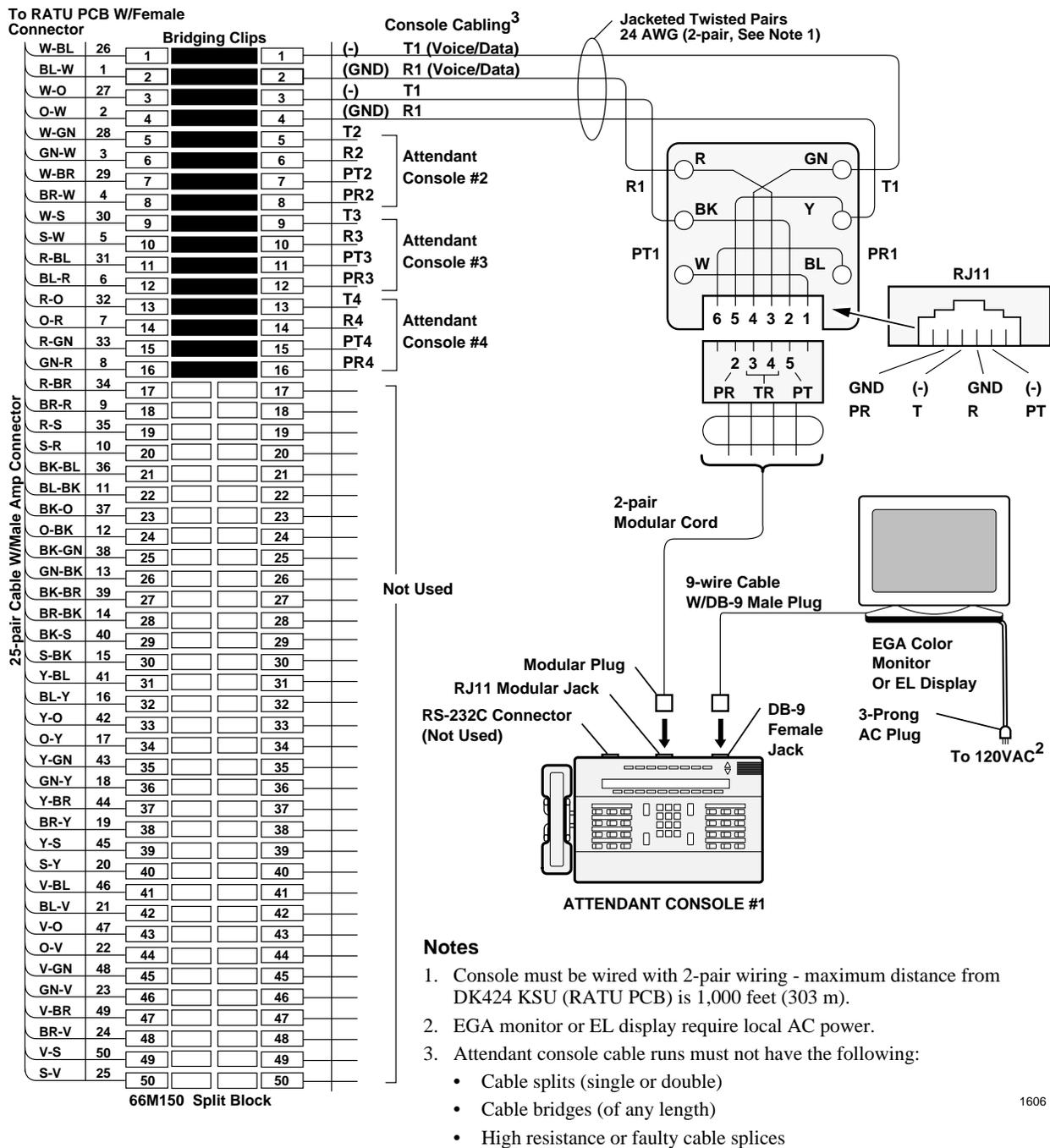
Figure 8-17 Attendant Console MDF Wiring Diagram
