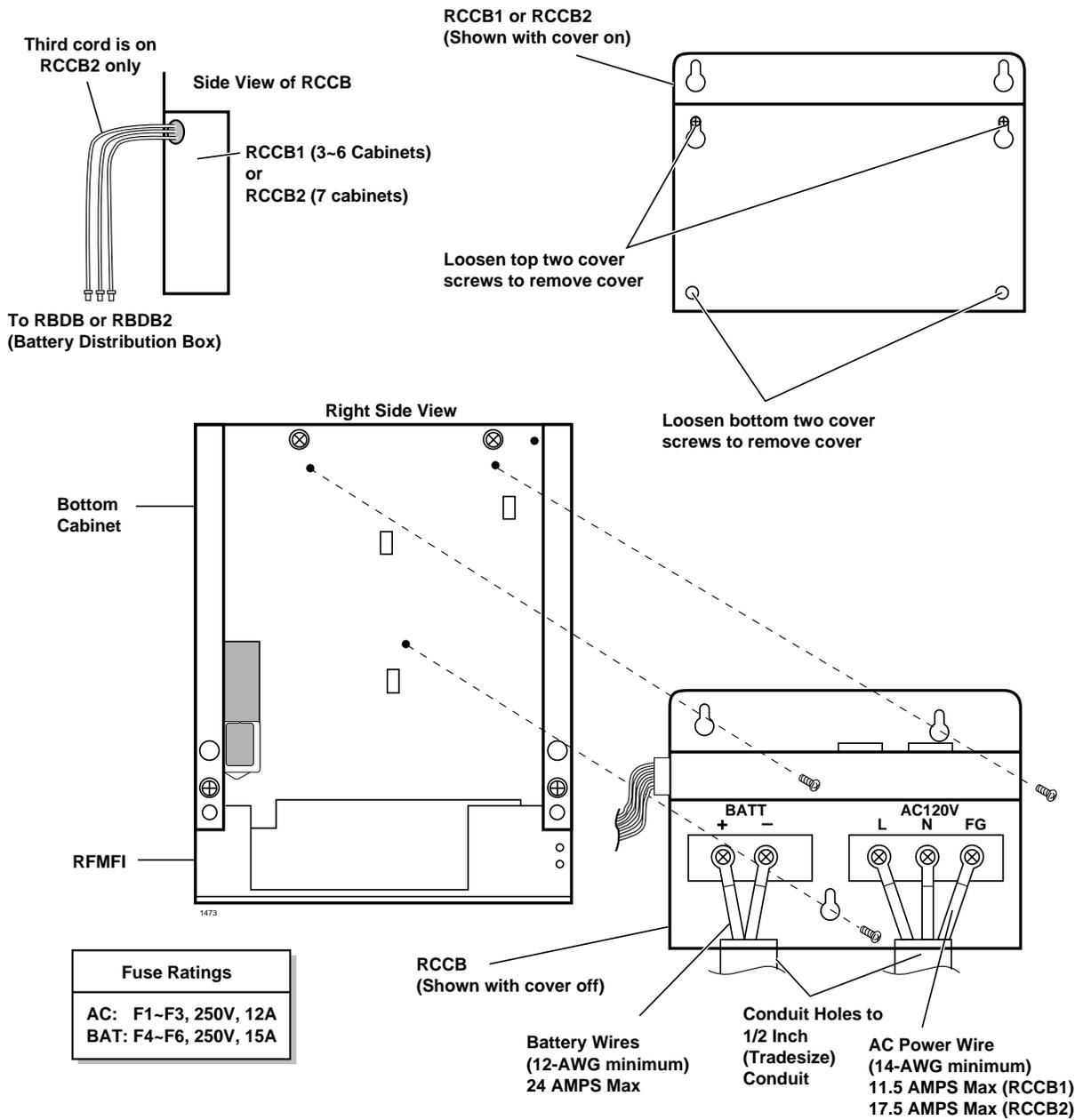
**Figure 5-26 Conduit Connection Box (RCCB)**
