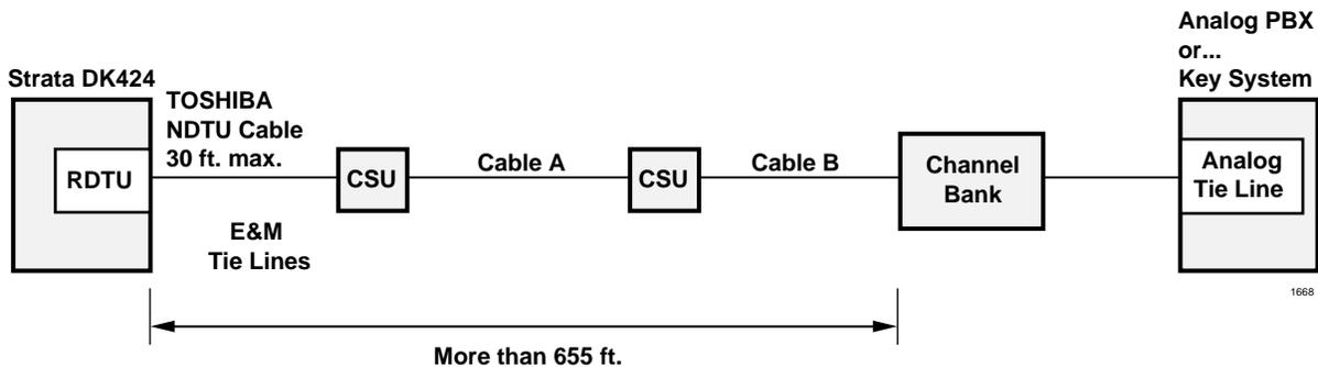
Figure 6-6 RDTU Connection via CSU and Channel Bank
