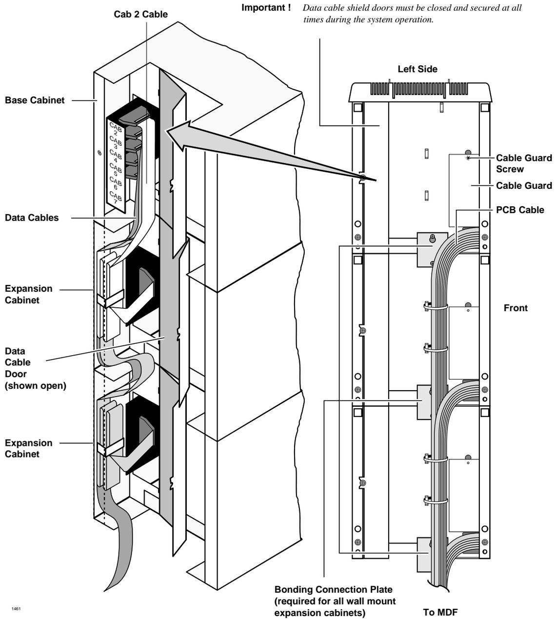
**Figure 5-10** Left Side View of Cabinet Interior
