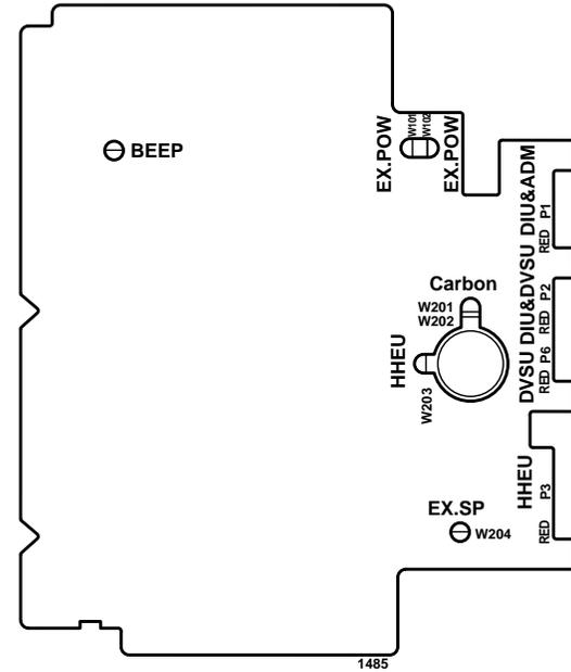
Figure 9-9 DKT2010-SD, DKT2020-S, and DKT2020-SD Strap and Connector Locations
