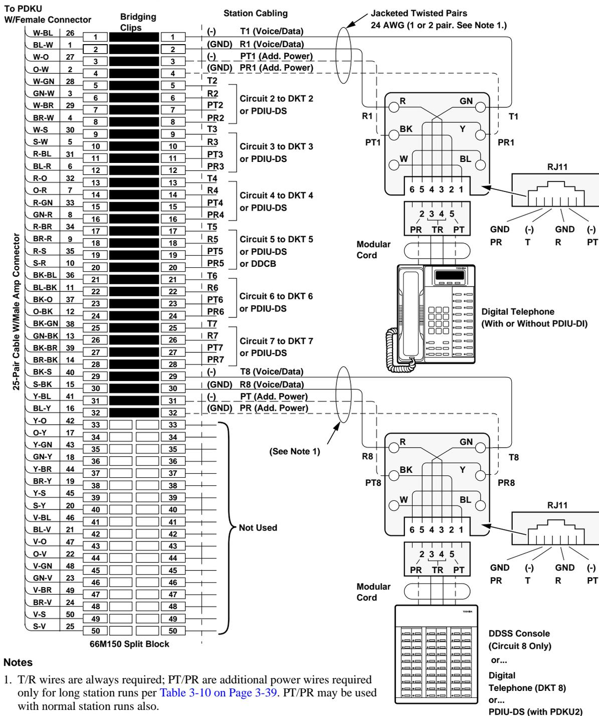
Figure 8-1 MDF Wiring for Digital Telephones (DKTs) and DDSS Console to PDKU
