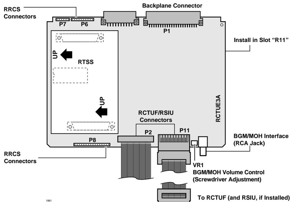
**Figure 5-37 RCTUE PCB with RTSS Subassembly**
