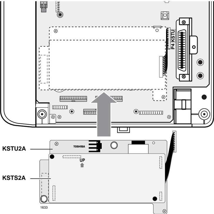
**Figure 3-19 KSTU2/KSTS2 Installation**
