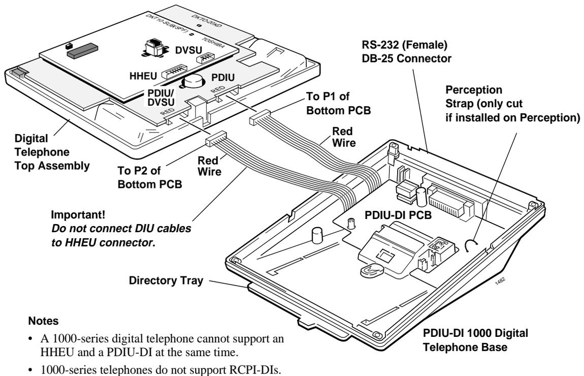
Figure 9-6 PDIU-DI Installation into 1000-series Digital Telephone
