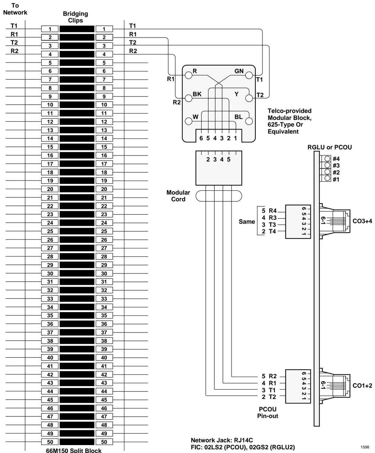
Figure 8-24 MDF Wiring/CO Lines to RGLU2 or PCOU
