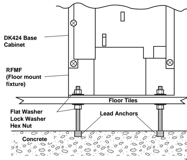
Figure 5-18 Floor Mount Installation – Computer Room Floor
