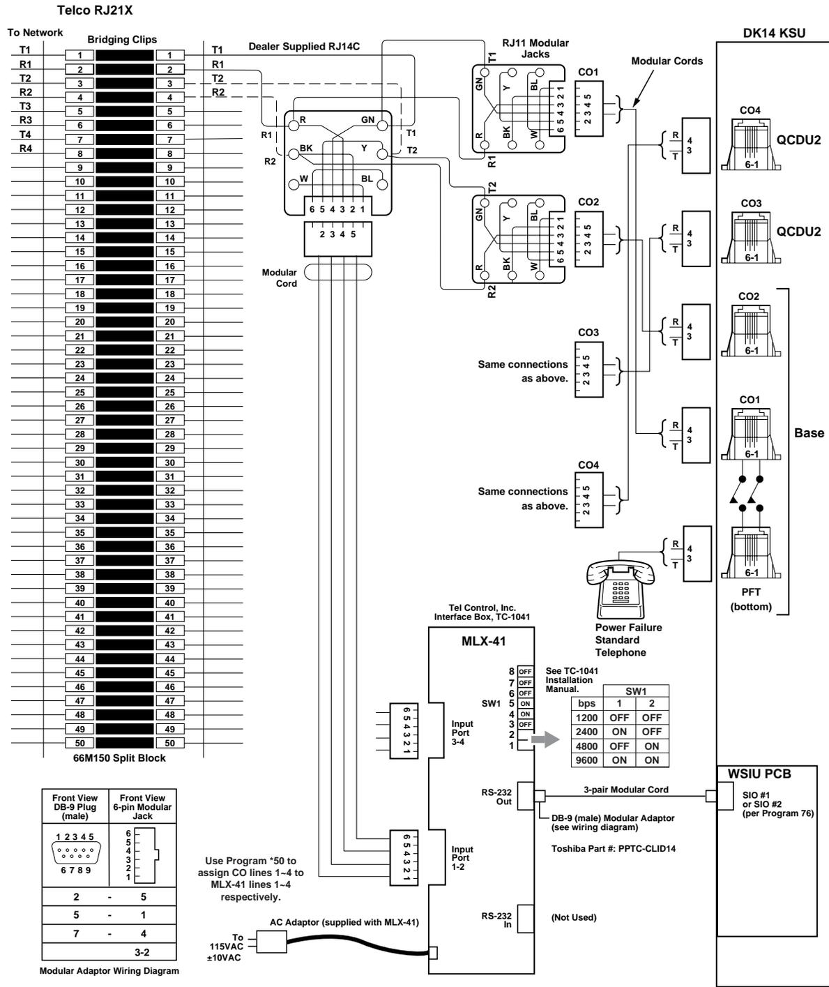
Figure 1-18 DK14 MDF Wiring to Caller ID Interface (WSIU)
