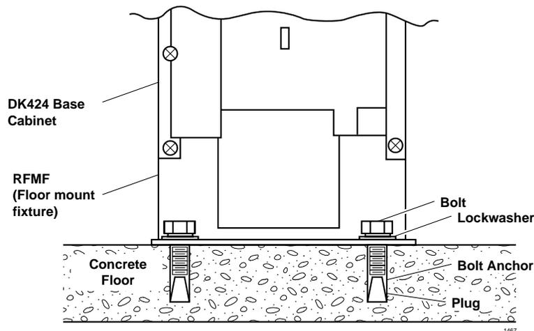
Figure 5-16 Floor Mount Installation – Concrete Floor
