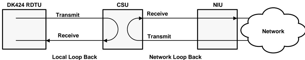
**Figure 6-3 CSU Local and Network Loop Back Tests**
