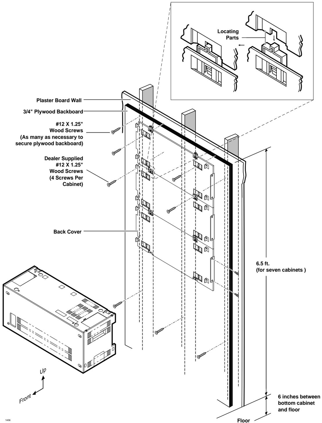
Figure 5-5 DK424 Cabinet Mounting Surface Diagram (with Plywood Backboard)
