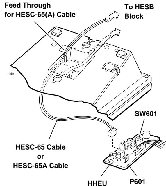
Figure 9-12 HESC-65A Cabling
