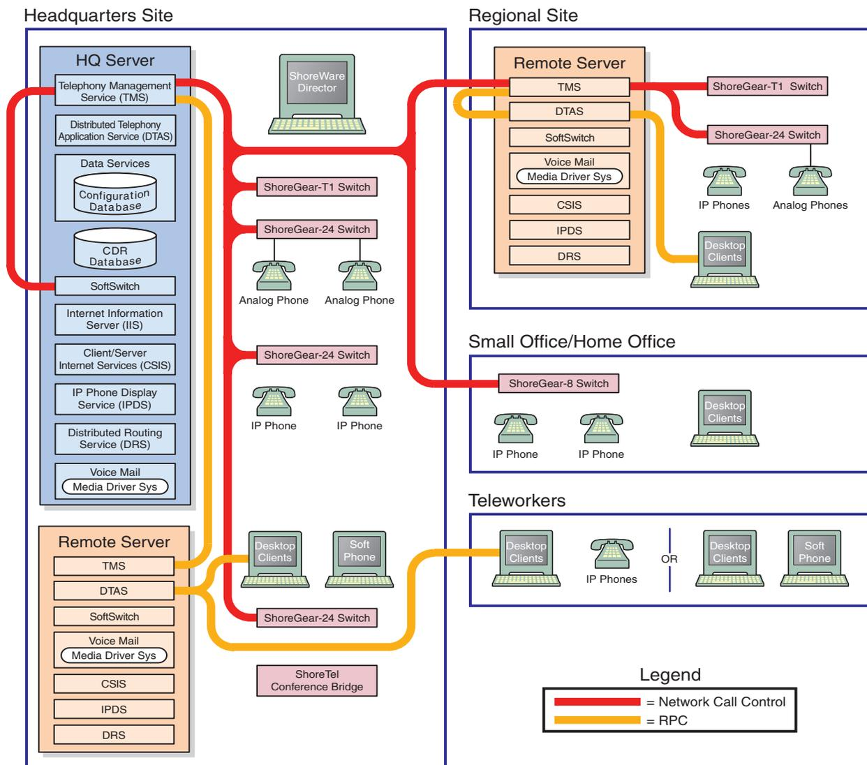
Figure 2-5 NCC and RPC Communications in a ShoreTel System
