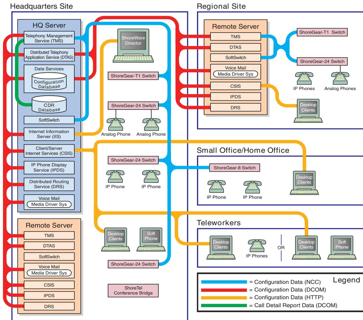
Figure 2-4 DCOM Protocol in a ShoreTel System
