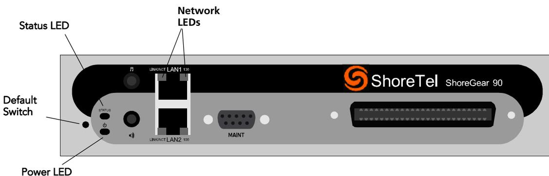
Figure 4-2 ShoreGear-90 LEDs
