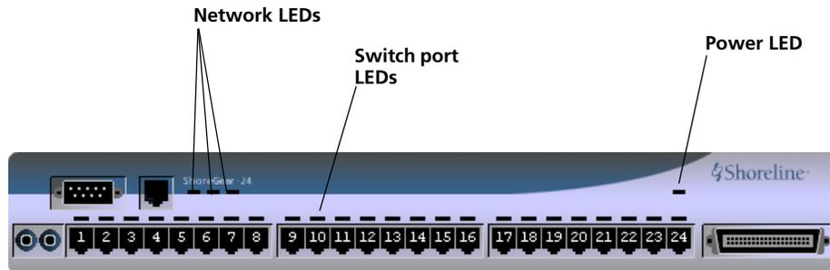
Figure 4-9 ShoreGear-24 (IPBX-24) LEDs
