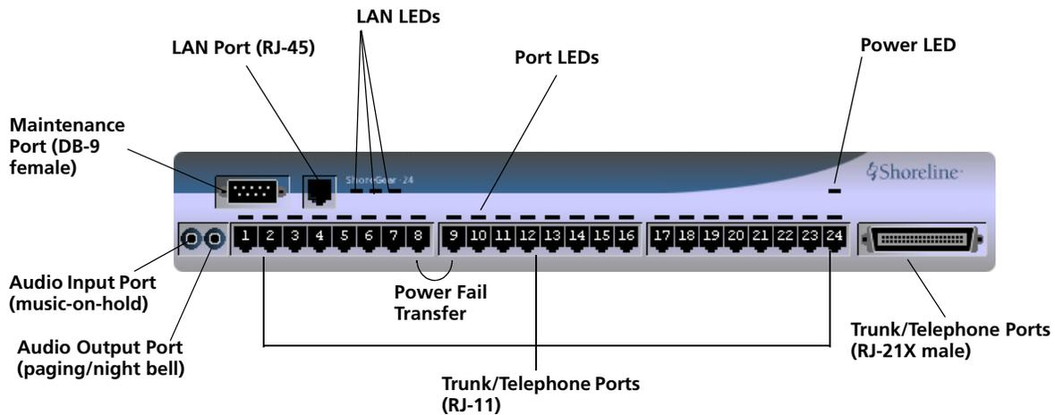
Figure 4-26 ShoreGear-24 (IPBX-24) Connectors and LEDs
