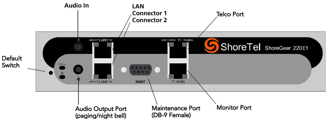
Figure 4-24 ShoreGear-220E1 Connectors
