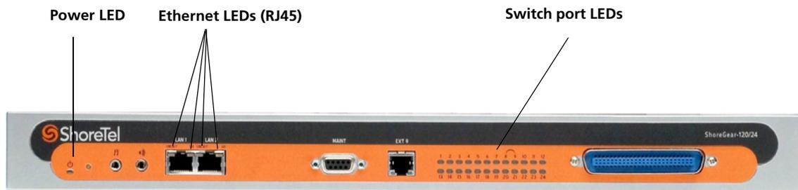
Figure 4-1 ShoreGear-120/24 LEDs
