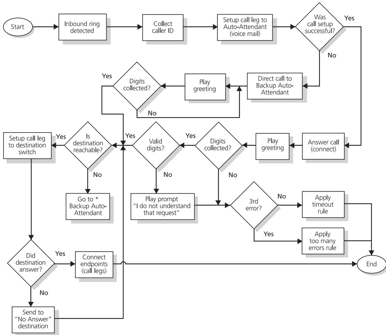
Figure 2-9 Call Flow for an Inbound Trunk Call
