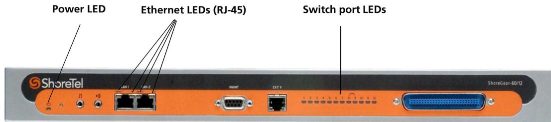
Figure 4-3 ShoreGear-60/12 LEDs
