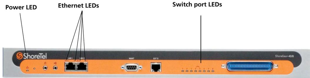
Figure 4-5 ShoreGear-40/8 LEDs
