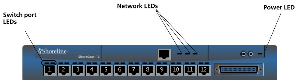
Figure 4-10 ShoreGear-12 (IPBX-12) LEDs
