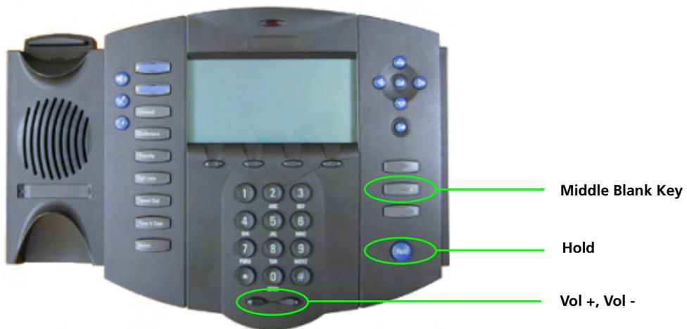
**Figure 5-1** Reboot Keys on the ShorePhone IP Phone
