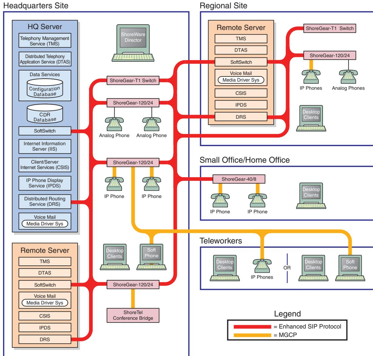
Figure 2-3 SIP and MGCP in a ShoreTel System
