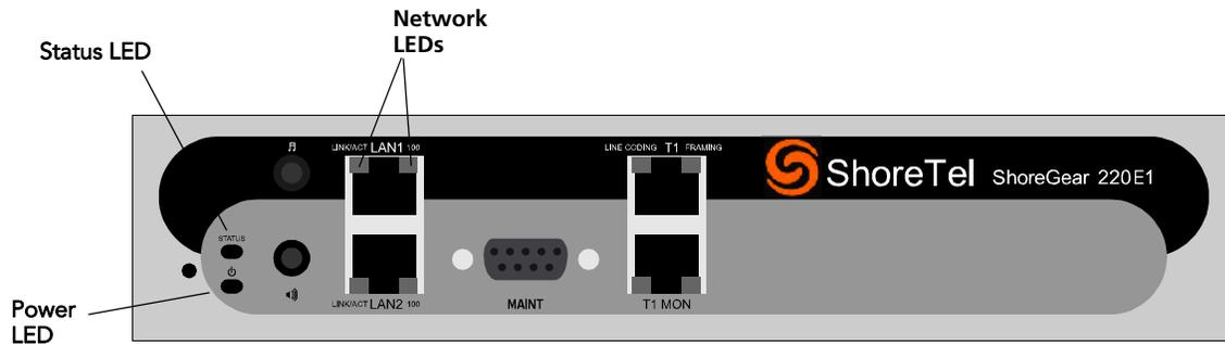
Figure 4-7 ShoreGear-220E1 LEDs
