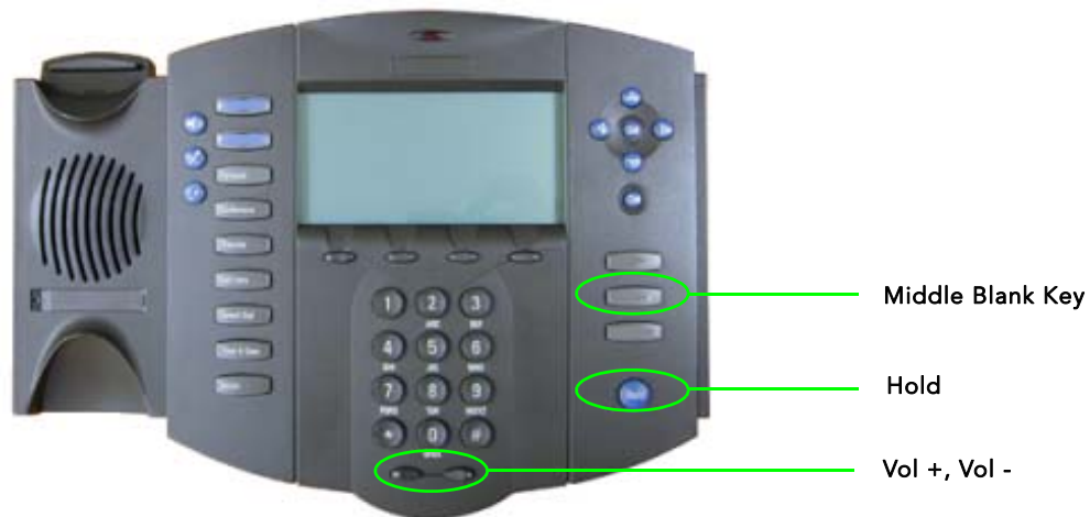
Figure C-1 Reboot Keys on the ShorePhone-IP100
