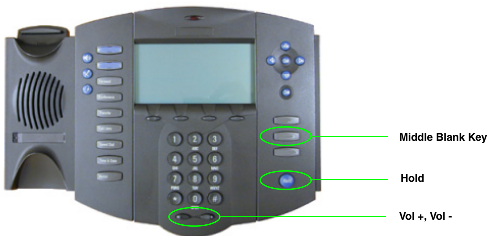
Figure 5-1 Reboot Keys on the ShorePhone IP Phone
