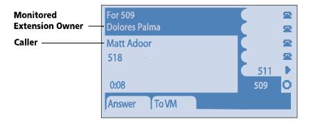
You can pick up the call while it is ringing by pressing the **Answer** soft key, or you can send it to the monitored extension's voice mail by pressing **To VM**. You can also answer a call after the owner of the monitored extension has put it on hold by pressing the **Pickup** soft key.
