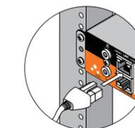
Use an RJ-45 Ethernet cable to connect one or both of the LAN ports to the network subnet.
