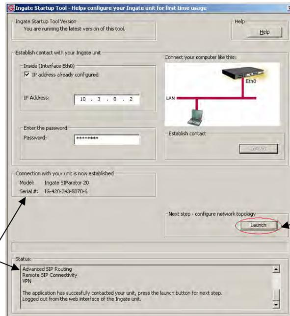
Once "contact" has been established, step two is to configure the Network Topology by clicking on "Launch".
