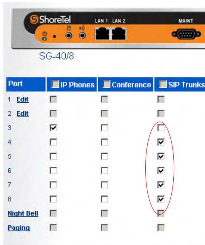
Figure 8 - ShoreGear Switch Settings
