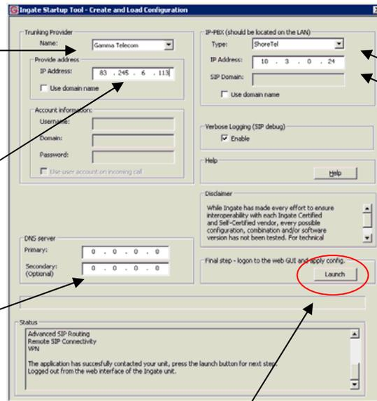
**D. Select ShoreTel from the drop-down menu and IP address of ShoreGear Switch Configured for SIP Trunks.**
