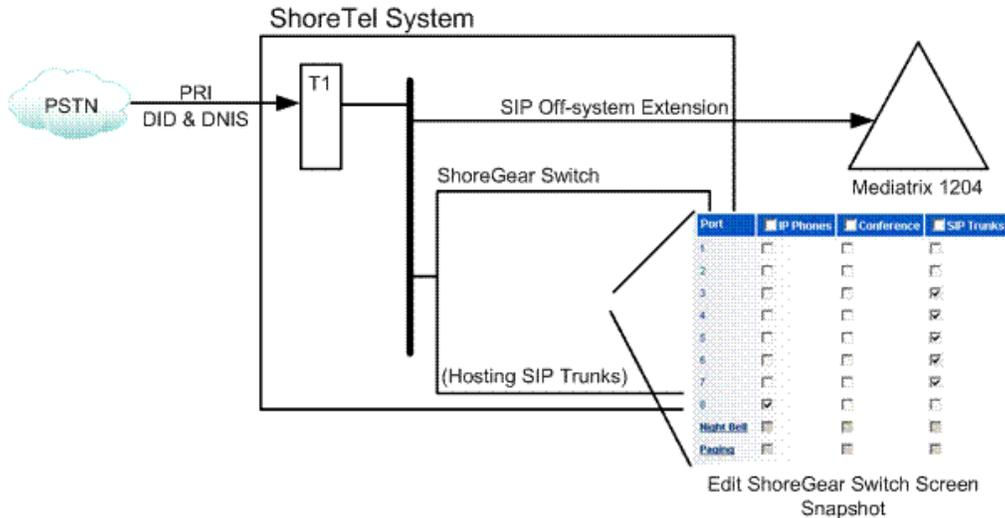
2. Routing through Individual User Extension with the Call Handling Mode set to forward (external
