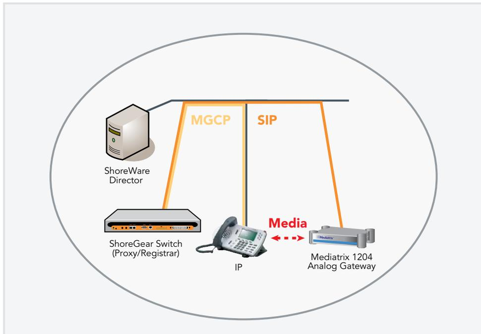
Sip devices are being implemented on the ShoreTel System with SIP trunks. The ShoreTel system will use outbound call routing for the SIP devices. There are various ways to handle the call routing for the SIP devices. The following drawings depict different call routing designs:
