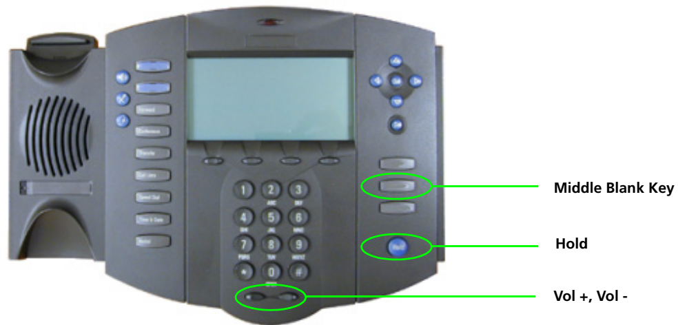
Figure 5-1 Reboot Keys on the ShorePhone IP Phone
