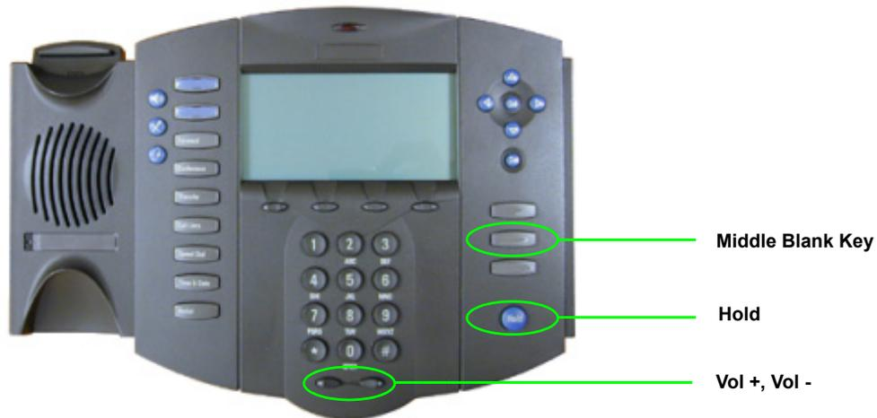
**Figure 3-1** Reboot Keys on the ShorePhone-IP100
