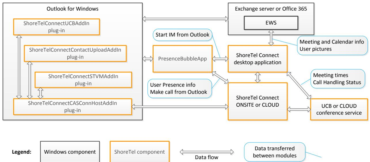
Figure 2 - Flow diagram for Windows
