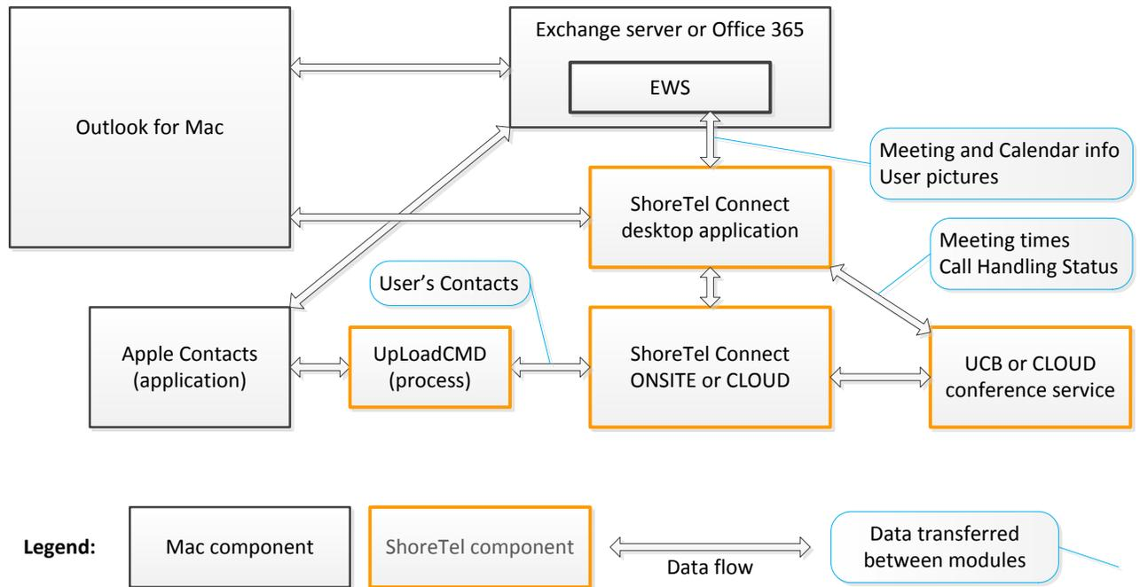
Figure 3 - Flow Diagram for Mac
