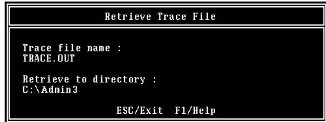
If you need a different directory, type over the default. Press **Enter**. Be sure to enter the complete path. If the directory already exists, you are given the option of entering a new directory or overwriting the file. The Trace Filter Setup screen displays (see [Figure 11-1](#) on [page 11-8](#)).
